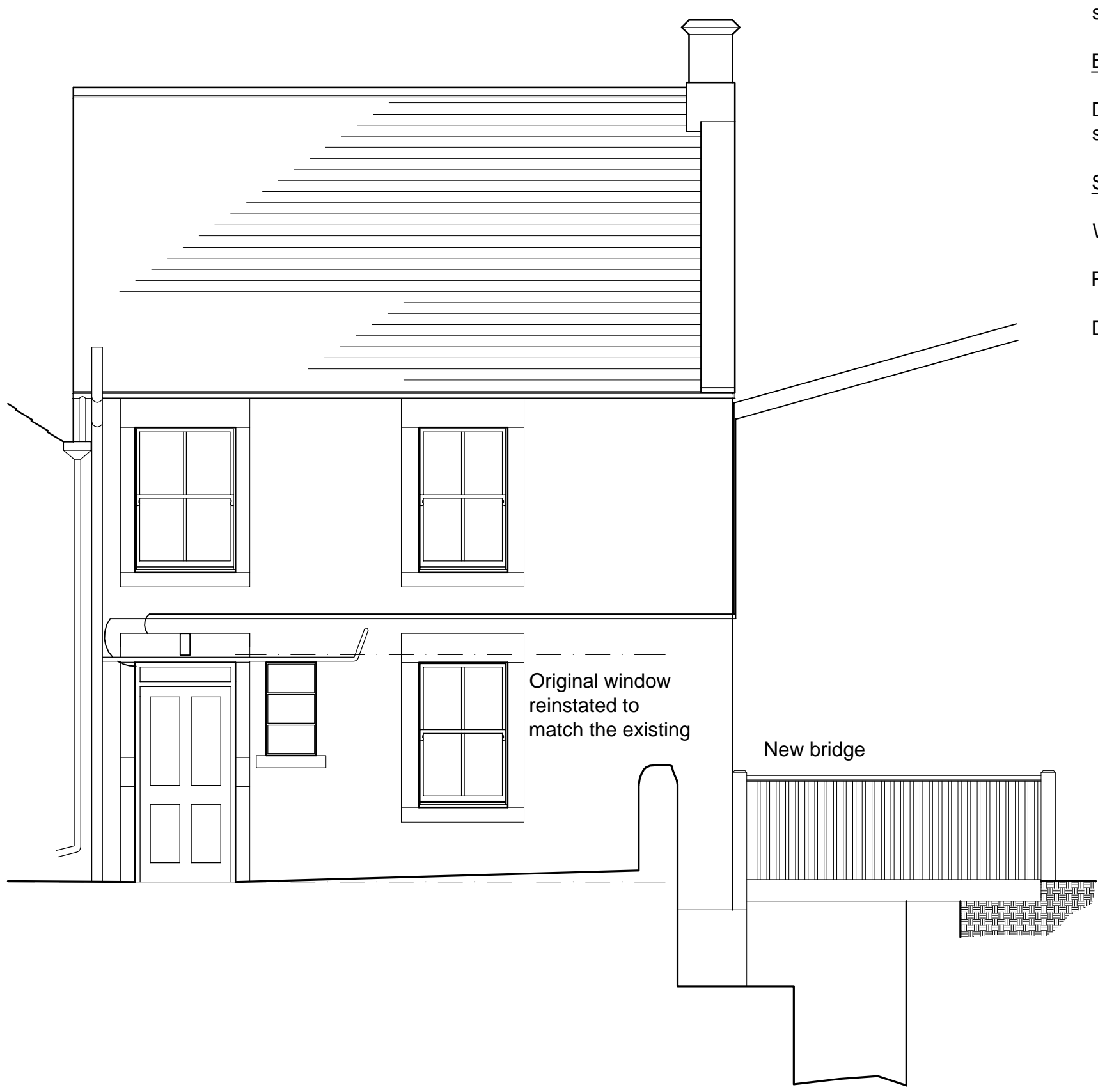
PROPOSED NORTH ELEVATION 1:50
